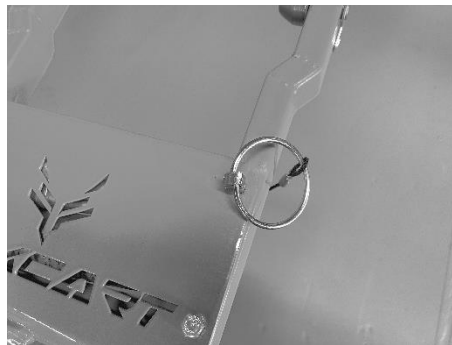
Safety pin on left actuator
